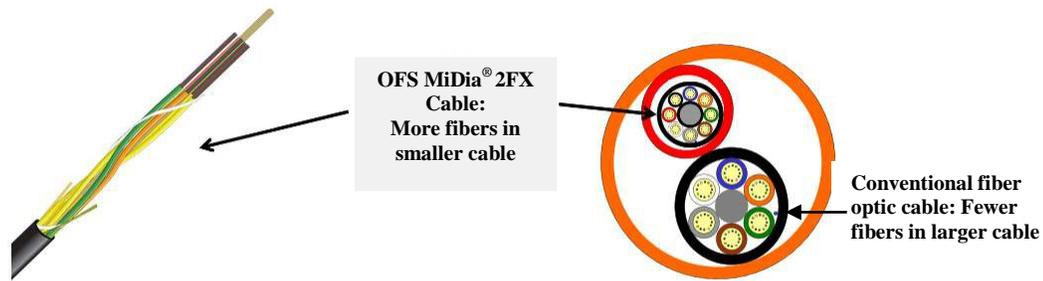
The figure above illustrates how microcables have evolved to feature twice the fiber density that was offered a few years ago. While both cables have 288 fibers, the conventional cable is 14 mm in diameter, while the newer design is 9.6mm. The new design takes advantage of the new 200-micron coated fiber and is 36 percent smaller than the traditional cable.
