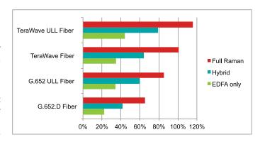
Expected regeneration distance at 400 G compared to standard single-mode fiber at 100 G using EDFA
